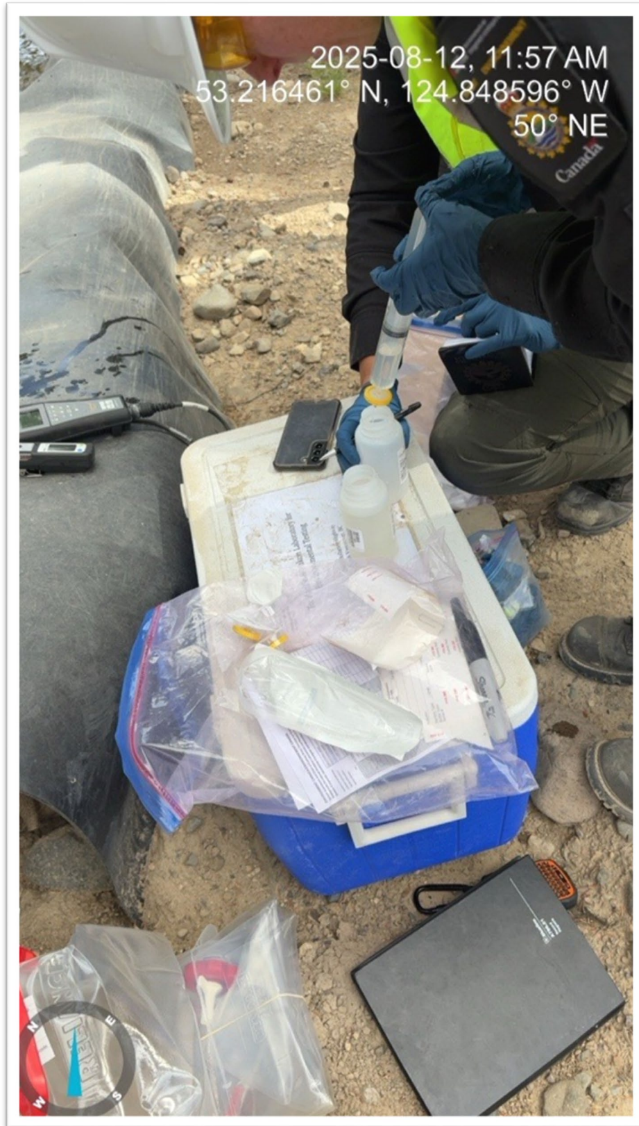
Photo 44: ECCC Filtering the Water Sample
