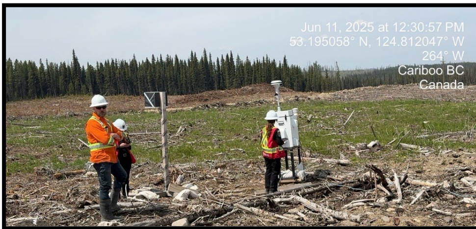
Photo 11 Partisol Air Quality Station
