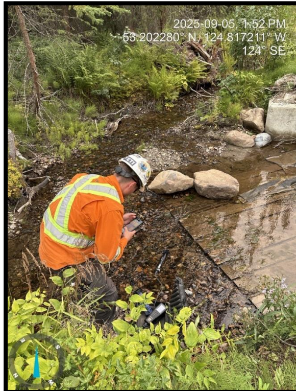
Photo 30: YSI reading at Creek 146 Job Structure
