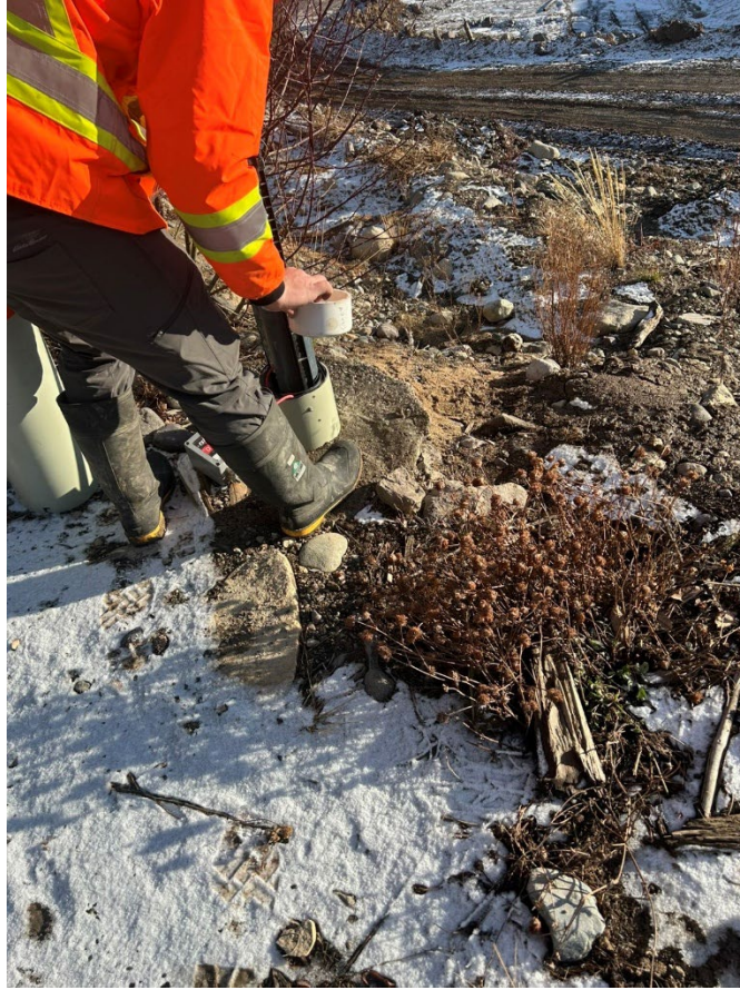
Groundwater well sampling
