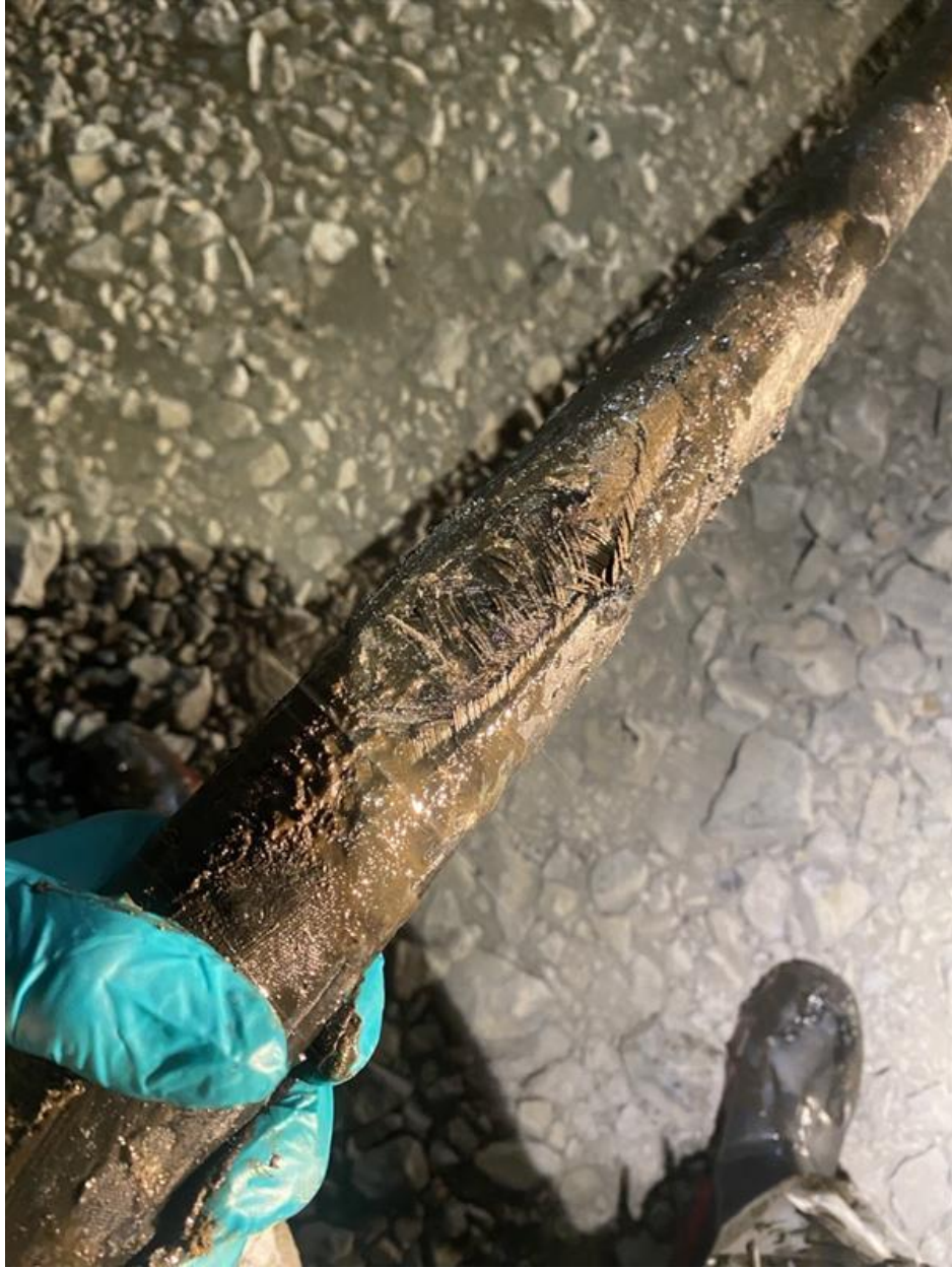
Photo 6: Hydraulic hose failure
