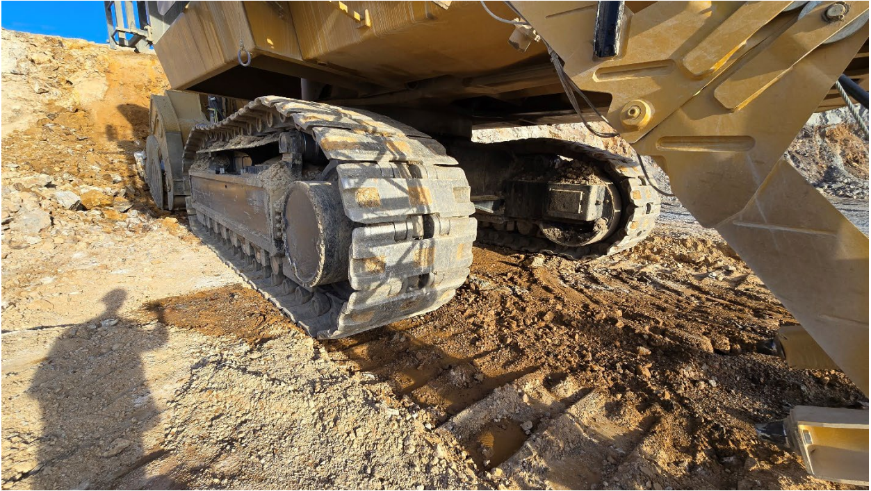
Photo One: Coolant Spill
