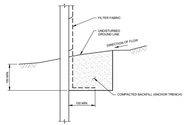
**SILT FENCING - CROSS SECTION**
