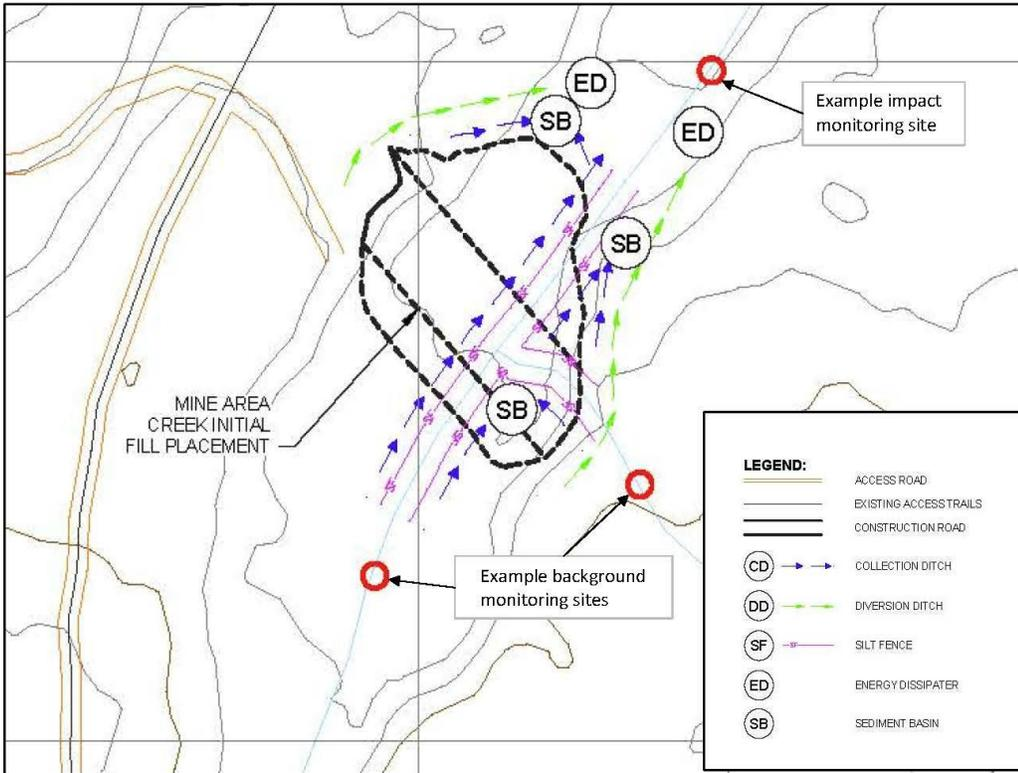
**Figure 1 Background and Impact Monitoring Location Example**
