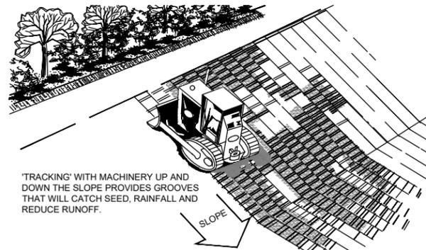
'TRACKING' WITH MACHINERY UP AND DOWN THE SLOPE PROVIDES GROOVES THAT WILL CATCH SEED, RAINFALL AND REDUCE RUNOFF.
