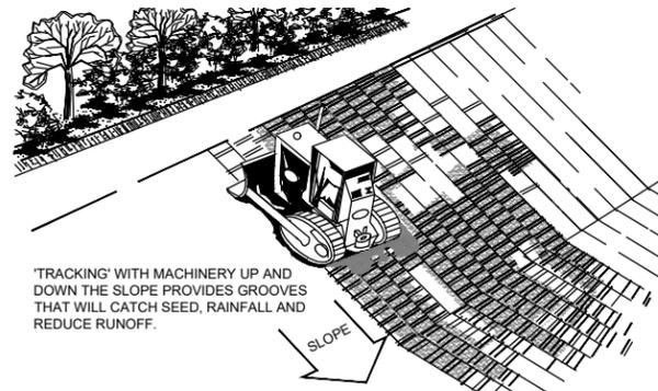
'TRACKING' WITH MACHINERY UP AND DOWN THE SLOPE PROVIDES GROOVES THAT WILL CATCH SEED, RAINFALL AND REDUCE RUNOFF.
