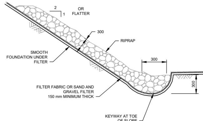
**AS ARMoured SLOPE - TYPICAL**
