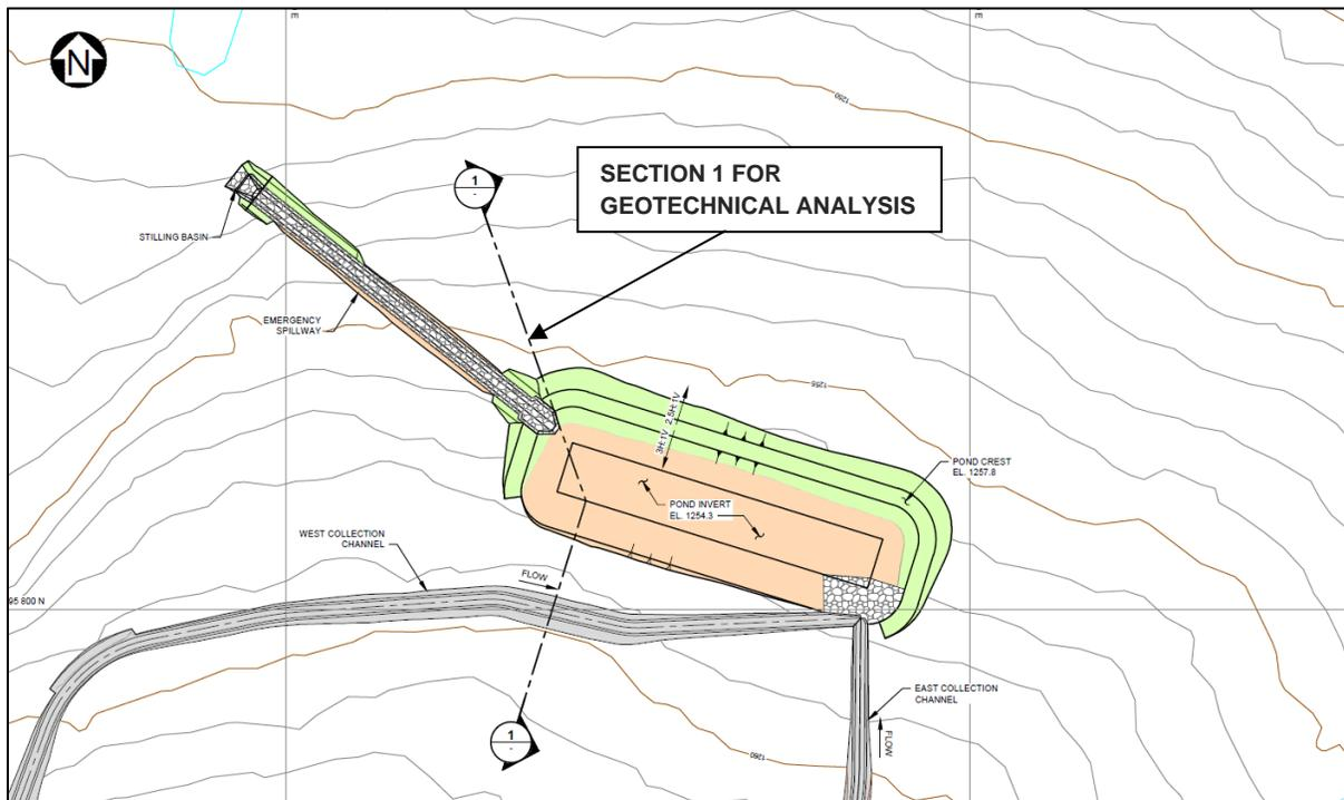
**Figure 7.1 Camp Site SCP – Plan and Section for Geotechnical Analyses**
