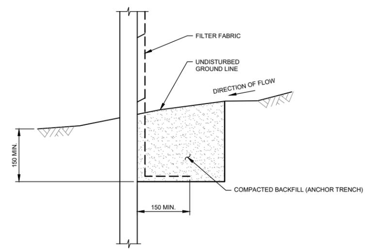
**SILT FENCING - CROSS SECTION**
