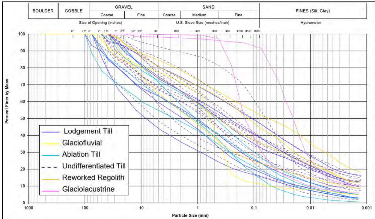
**Figure 3 Plant Site Samples – Particle Size Distribution**
