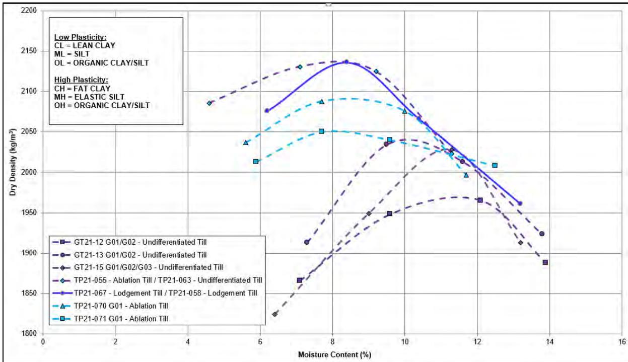
**Figure 5 Plant Site Samples – Compaction Data**
