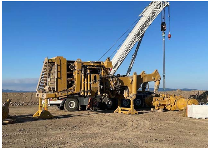
CAT 793 production haul truck to be assembled on site
